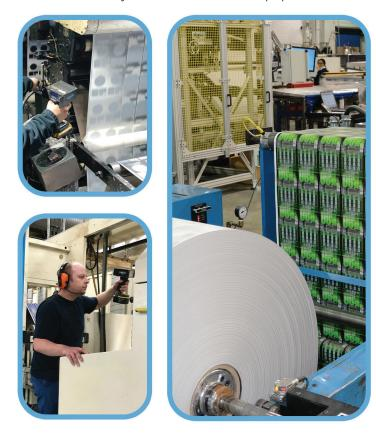
The back of the ticket is printed, and then multiple security layers are laid down, beginning with a lower opaque black security coating that provides good adherence to the paperboard and prevents light penetration. Next, a white or tinted security primer is applied over the black coating to create a secure, image-receptive play area. The ticket is now ready to receive the game data.
